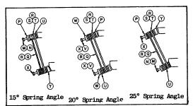
2. Remove all clamp bolts (M,V,X), blocks (W), wedges (N,Y), spacers (U) and leaf springs (P,Q,R,S,T).
